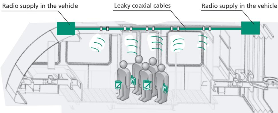
1 Leaky coaxial cables installed in the AutoTram® for radio propagation and positioning.
