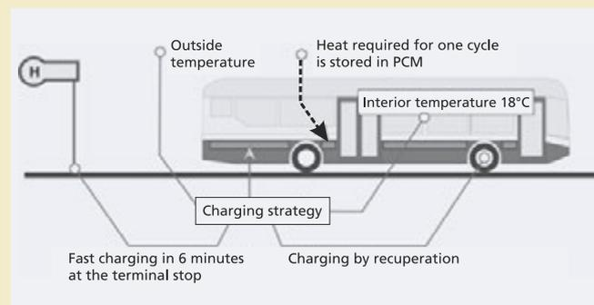
1 Operational principle of a fast-charging latent heat storage system.
