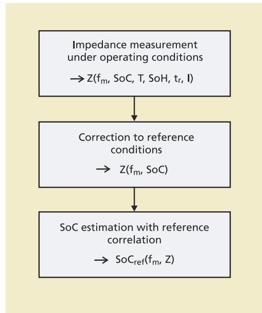
**1** State of Charge estimation based on battery impedance.
