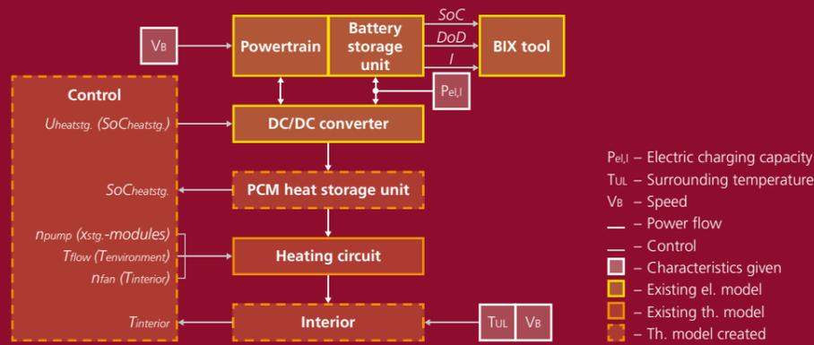
1 Simulation model of electric bus with sub-models.
